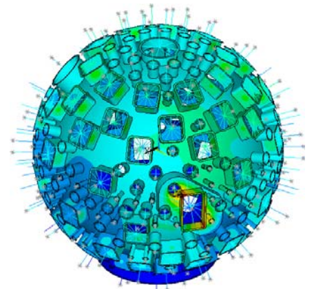
Design and calculation of the vacuum chamber for a fusion Laser MegaJoules experiment (CEA)
