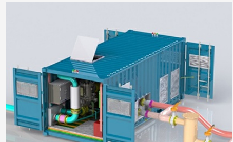
EDF - Mobile cooling modules for spent fuel pools (PTR Bis)
